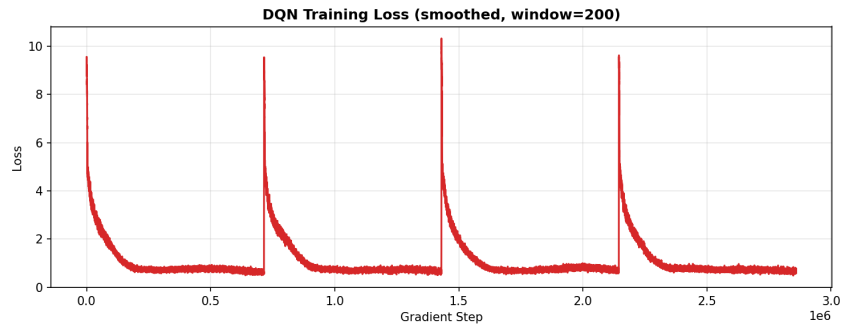
Figure 14: DQN training loss (Huber / Smooth L1, smoothed; four seeds concatenated). Each spike marks large-magnitude night-violation penalties ( -30 ) entering the replay buffer, followed by a monotonic decay as the target network stabilises.
